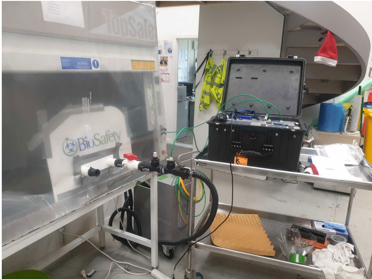
Decontamination Validation Set Up – Sealed BSC with recirculation blower, EMS real time gas monitoring
