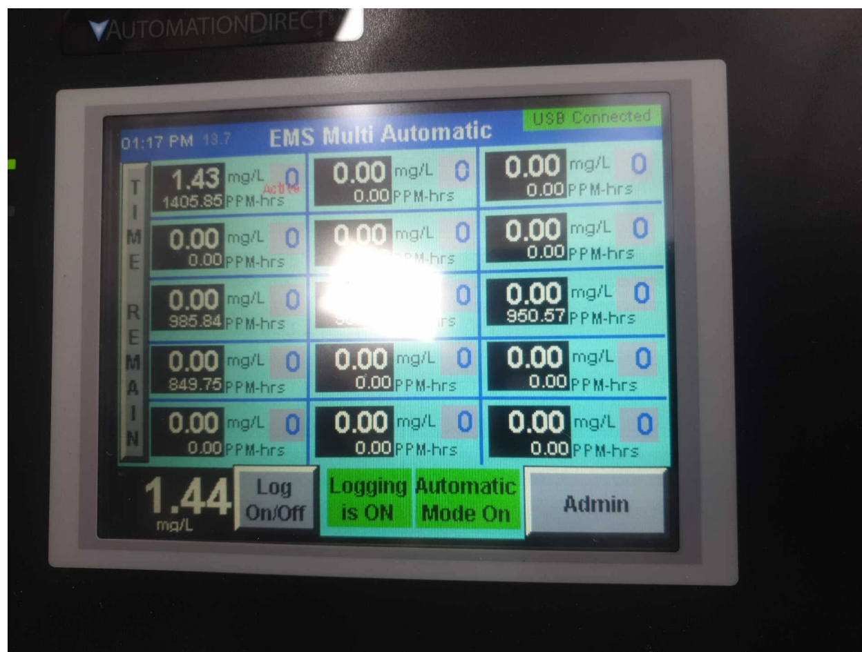
Exemplar EMS monitoring screen. Top left cell demonstrating 1.43 mg/L current concentration, 1405.85 ppm-hrs total accrued exposure
