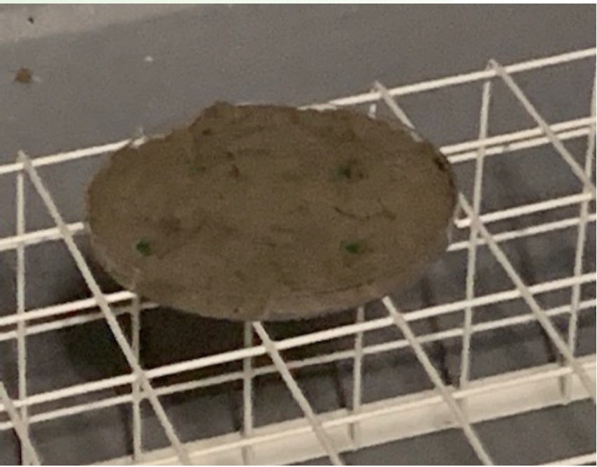
Figure 3. 4mm of dust covering BI, showing dust and debris penetration of chlorine dioxide gas.
